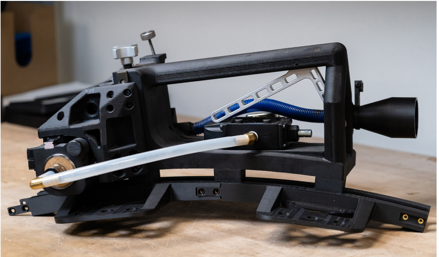
This printed MRO tool from the Siemens Energy Innovation Center mitigates 3-4 weeks of downtime per instance. Both prototypes and final end-use parts can be printed, leading to significant time and cost savings.
