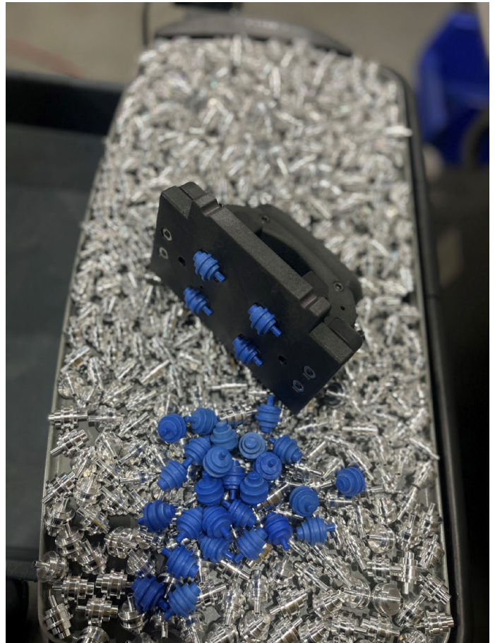
Custom tool used for manually loading brass inserts into injection molding machine.
